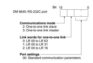
**Communications Procedure** If the settings for the master and the slave are made correctly, then the one-toone link will be automatically started up simply by turning on the power supply to both the C200HSs and operation will be independent of the C200HS operating modes.
